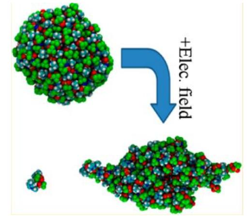
Classical MD simulations of EMIM NTf<sub>2</sub> nano-sized droplets under electric fields [2]
