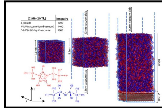
Fundamental study of EMIM NTf<sub>2</sub> in the bulk, liquid-vacuum interface, and liquid-solid interface [1]
