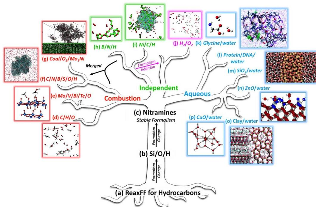
Iterative methodology of ReaxFF force field MD simulations (left) and ReaxFF development tree, where each branch represents a transferable set of parameters for hydrocarbon applications (right) [1]
